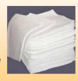
Oil Absorbent Pads: MeltBlown Mat, Sonic Bonded & Fine Fiber Pads quickly absorb oil for effective cleanup of petroleum-based spills on land or water. Polypropylene fibers are left in their natural hydrophobic state. These hydrophobic fibers repel water while only absorbing oils and other hydrocarbons.
