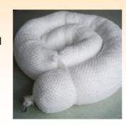
Oil Absorbent Boom: Strong mesh outer sleeve encases a poly sock skin filled with highly-sorbent polypropylene. Filler won't shed and Booms won't sink, even when saturated with oil. A nylon rope and sturdy hardware ensure long-lasting durability and easy retrieval. Durable, easy-to-use connectors provide a simple and efficient way to link Sock/ Net Booms together and create a containment system big enough to handle almost any size spill on water. Clip together with metal connector hardware.
