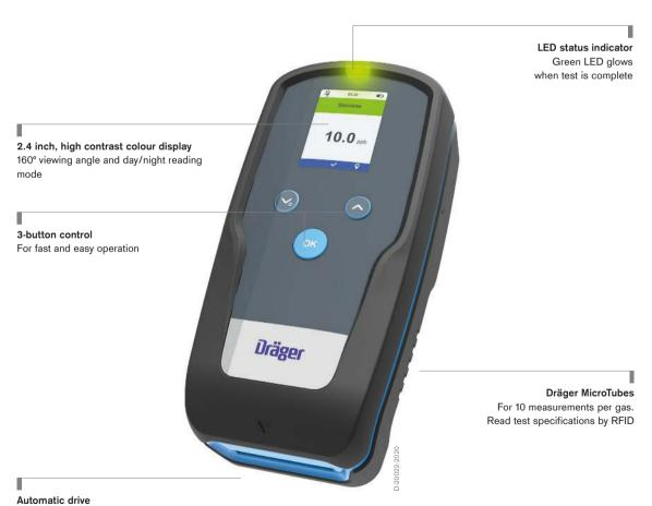
For retracting the Dräger MicroTubes
